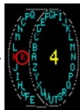
Ring Offset to Rotor
