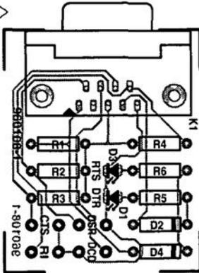
**Figure 2. Track layout and component mounting plan of the printed circuit board designed for the project (board not available ready-made).**
